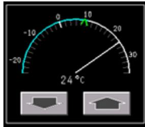
Figure C-1.1 – Cabin Temperature DU Window
