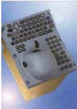
Figure 1. KCCU (Keyboard Cursor Control Unit) for interactive cockpits taken from A WST (September 27th 2004)
