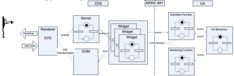
Fig 1. Detailed architecture to support ARINC 661 specification
